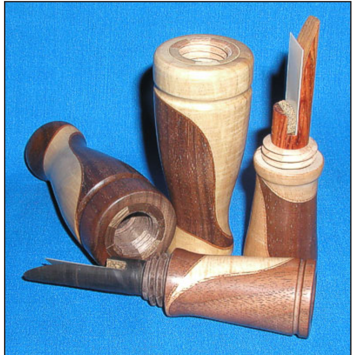
This matched set of wedge pattern calls sports threaded inserts between the barrels and stoppers, replacing the traditional friction fit between the two.
