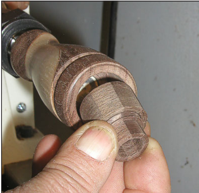
Test fit the female insert in the barrel to assure a snug fit. Fit the male insert in the stopper the same way.
