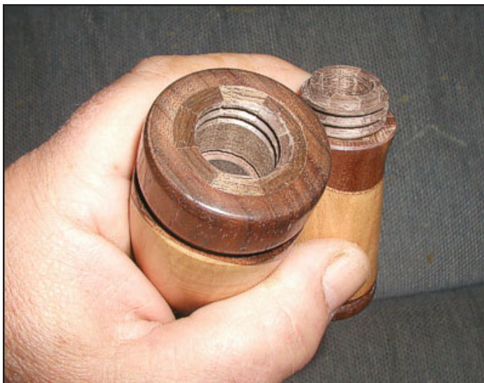
The inserts are fitted and glued in place. The outside is finished here, the inside of the call, including the threads will receive a tung oil finish.
