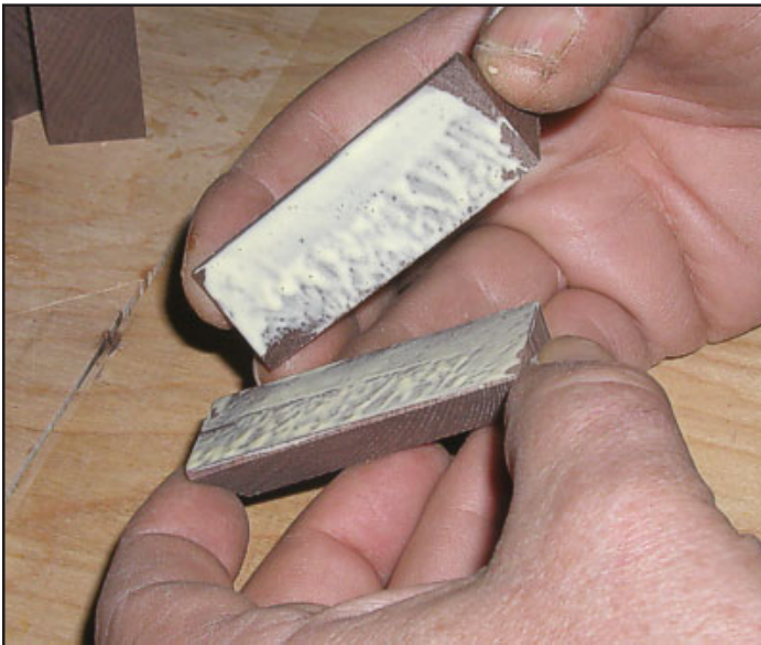
When gluing parts like this, rub the parts together to spread the glue over the entire joint.
