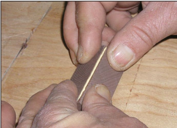
Rub the parts back and forth with increasing pressure to achieve a uniform squeeze-out. The glue will eventually squeeze out until you get a "tack." Hold the pieces a few more seconds and then you can set the pair aside to cure.
