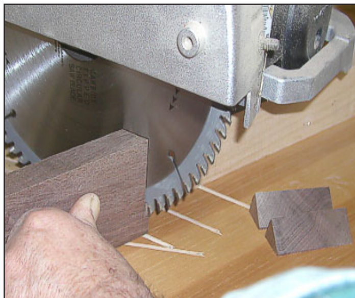
Chopping the segments cross grain will mean the threads will be cut running with the grain all around the assembled segment. Note the tiny flat left on the inside of each segment.
