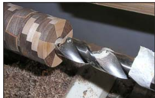
Fig. 21 I counter bore the stopper end of the barrel .75" x 2.75" deep to receive the stopper and to create a resonance chamber. The barrel's mouth piece remains at .5"
