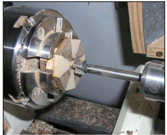
Fig. 17 I mount each group of rings in a spigot chuck, a drill chuck in the tailstock and bore .5" prior to final assembly.
