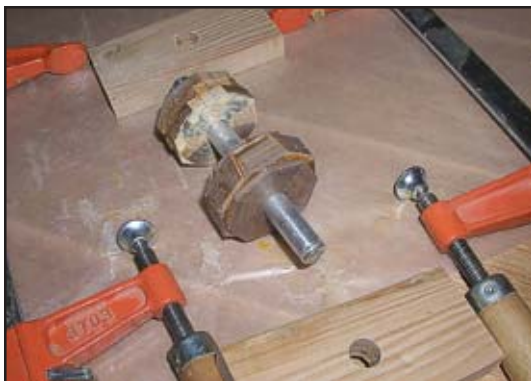
Fig. 18 Spread glue on groups of rings as you thread them on the .5" rod much the same as the glue up of rings into groups.
