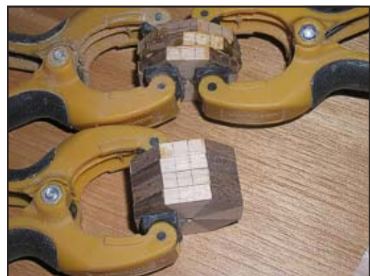
Fig. 15 When gluing rings into groups, mark the offset on three side of the rings to aid in getting the rotation even all around.
