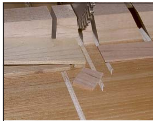
Fig. 11 The cherry dividers are cut square to the fence but we maintained the 10^{\circ} bevel from cutting the feature ring segments.
