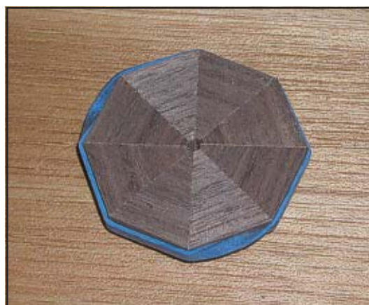
Fig 9 Segments should fit exactly to form a complete circle. Note the small hole in the center that aids in alignment of the segments and an escape route for glue squeeze out.
