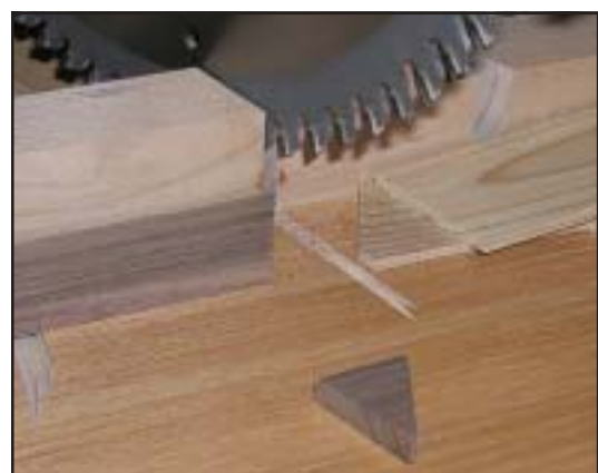
Fig. 8 Here you see the walnut strip ready to be pushed to the stop just to the right of the saw kerf in the auxiliary table. The springy hold down has been moved out of position to show the stop. To function the hold down must be near the saw blade as it cuts the segment. A chopped segment is in front.
