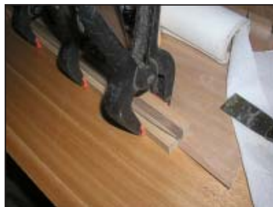
Fig 7 Use a pair of cauls and spring clamps to glue a strip of cherry to one side of the .5" black walnut. I pull the waxed paper up between the cherry and the outer caul to keep from gluing them together.
