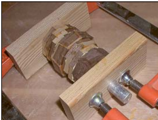
Fig. 19 The final assembly of the stopper includes three ring groups plus the ring that will insert in the barrel. Let the glue cure a few hours before turning.
