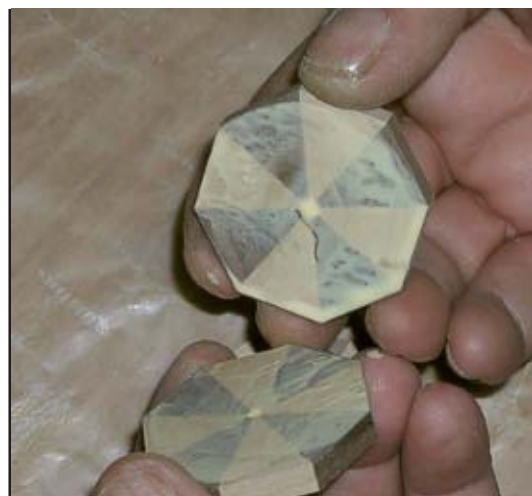
Fig. 16 When gluing rings together, make sure the glue is spread uniformly over the glue surface.
