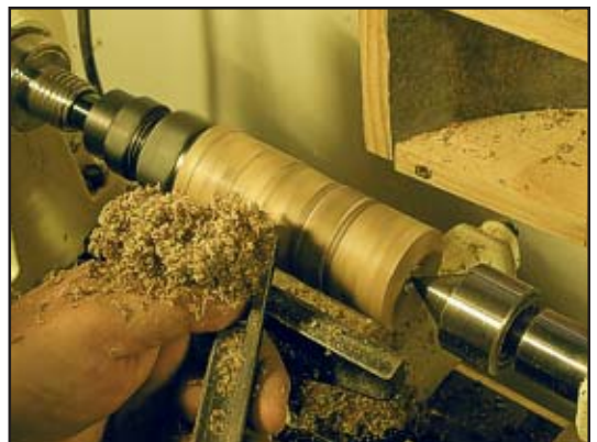
Fig. 20 Rough turn the barrel to its largest diameter. We'll remove it from the rod, chuck it in the spigot chuck and counter bore the stopper end.
