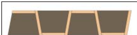
Fig. 3 The “Aztec” feature ring is composed of .5” thick black walnut alternately bordered and divided by .0625” cherry. The sides of each segment are chopped at 80° rather than the 90° chop used in “Southwestern Pottery.”
