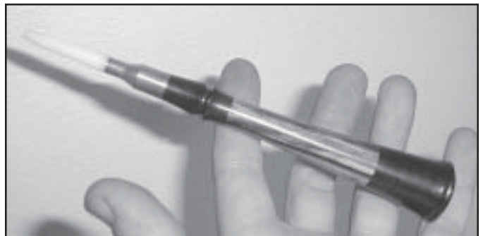
Scott's completed trumpet awaiting several coats of finish and the customer's preference for a lip stop. Scott doesn't use a lip stop but many customers specify one and Scott can add one of several designs from several different materials.
