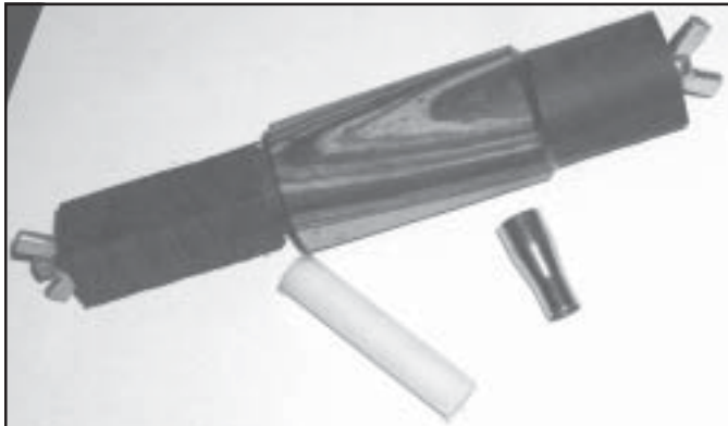
Three blocks, Gaboon ebony, black and white ebony and another Gaboon are glued with a threaded rod and wingnuts for a clamp. This trumpet will have a rifle shell ferrule and an ivory mouth piece.
