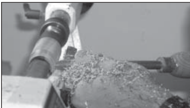
Turning begins with a pen mandrel and Scott has ground this spindle gouge to work like a scraping tool.
