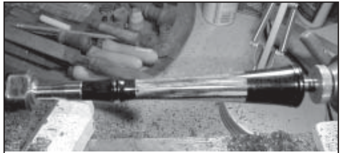
Turned to an precise outside diameter, this trumpet will now have the bell opened up. Then it will be fitted with an ivory mouth piece and when finished will be signed inside the horn.
