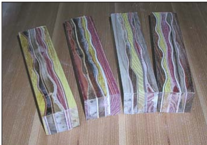
After four cuts, your blanks should look like this. Each blank will have the same wood on the outsides with the other three woods in different order on the inside. Note the randomness of the undulating cut lines.
