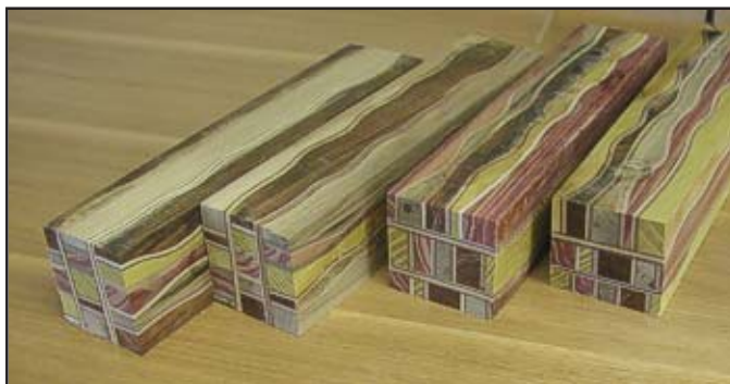
After the sixth cut is glued, the four blanks will look like this. Notice the "named" wood of each blank now only appears on each corner, most of which will be turned away in rough out.
