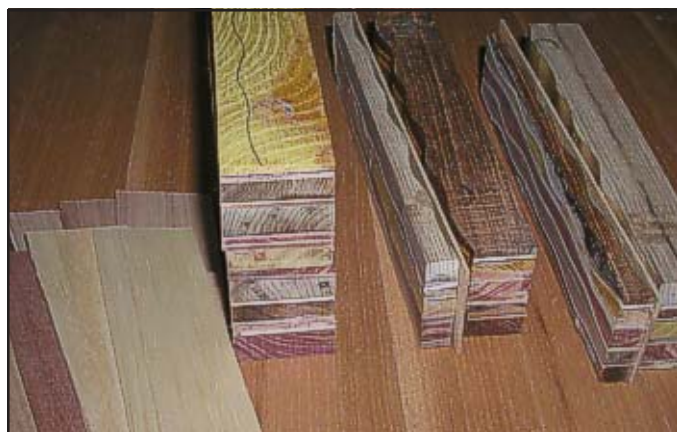
For the fifth (and sixth) cuts, the blanks are turned 90 degrees. The Osage and Tulip blanks at left are ready to clamp and cut while the two blanks at right have been cut and are ready to glue. You'll probably spend more for the broad selection of veneer strips (left) than for the solid wood blanks.
