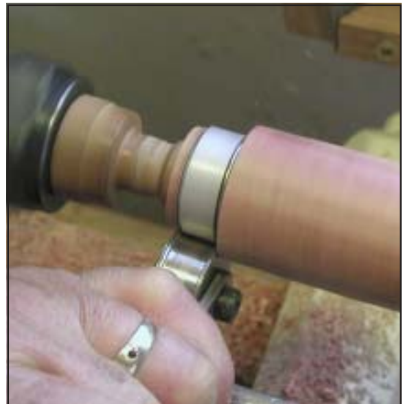
Fig 10 With the Ringer in place, it only takes 30 seconds to install a band.
