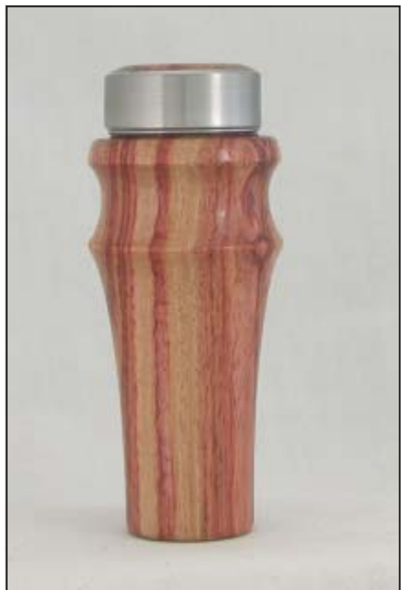
Fig 12 The finished barrel still shows the Ringer's shoulder marks but they can be turned or sanded.
