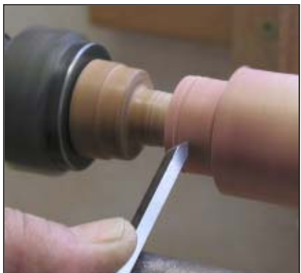
Fig 8 Cut the V-grooves to receive the Ringer's flanges and the rolled metal from the edges of the band.
