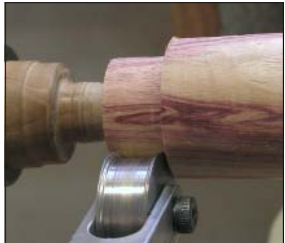
Fig 7 Use the Ringer to mark the position of the V-grooves
