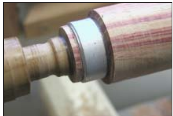
Fig 11 You need only roll about half of the band's wall thickness.
