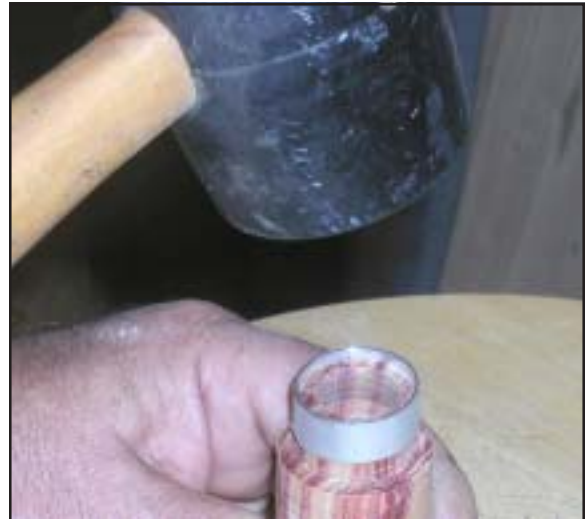
Fig 9 Drive or press the band on the blank's tenon.
