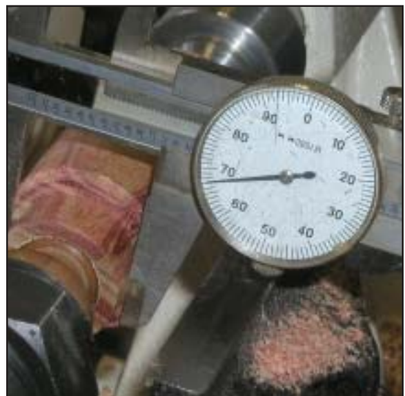
Fig 5 Turn the tenon a bit oversize.
